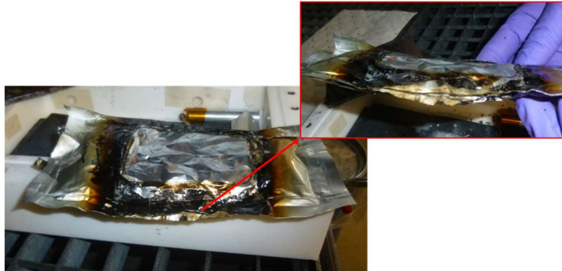
Figure 47 The post-mortem view of the cell left side: the tear on the bottom-left side of the cell can be clearly observed
