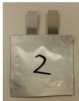
Figure 2: a) Uncontacted stack of cathode and anode. b) Electrodes after ultrasonic welding of tabs. c) Ultrasonic welding device. d) As-sembled pouch cell.
